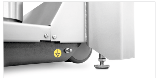
Electrical extensible supports to fix the table
